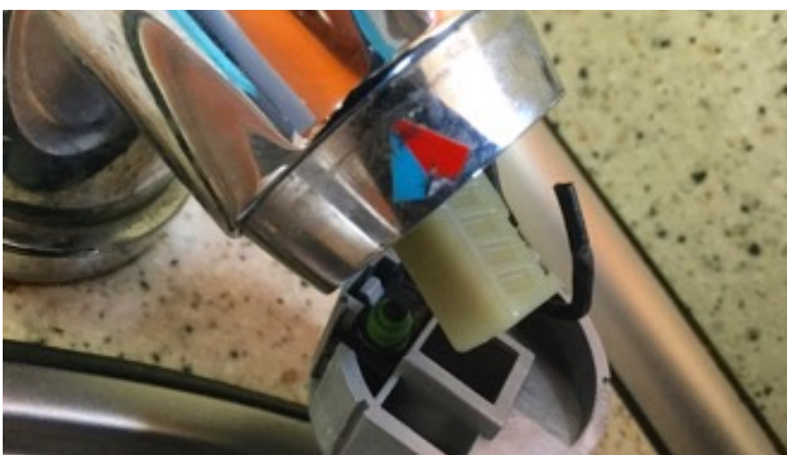
Nowhere for the wire to move so it rocks back and forth and twists with each tap operation until the wire breaks.
