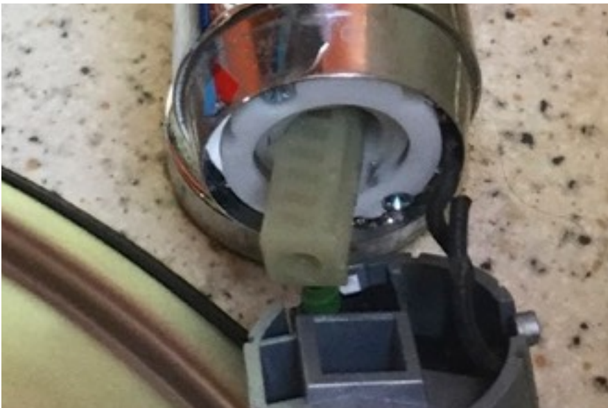
Access to the taps inside is via one clip at the rear of the tap and then one screw.
