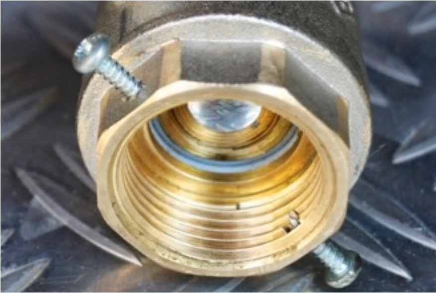
Above is the large valve, The edges filed down a little and then drilled to take a couple of self tapping screws
