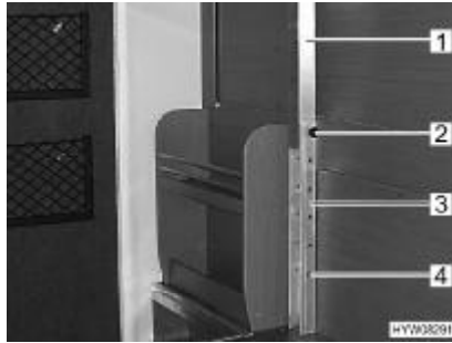
Fig. 67 Rear bed, mechanically lowerable
