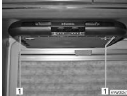
Fig. 142 Unscrewing the lower cover
