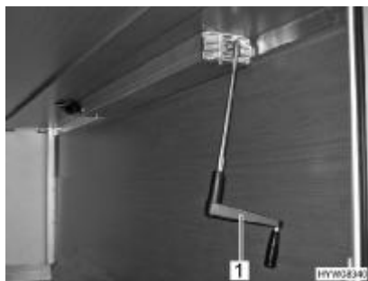
Fig. 68 Rear bed, mechanically height-adjustable
