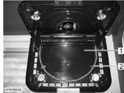
Fig. 143 Removing the grease filter
