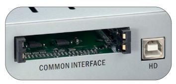
At the front of the device there are two slots for modules to decode encrypted programs.
